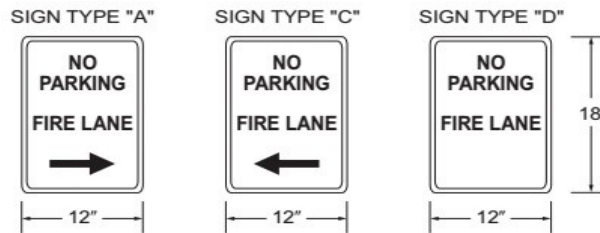
FIGURE D103.6 FIRE LANE SIGNS
