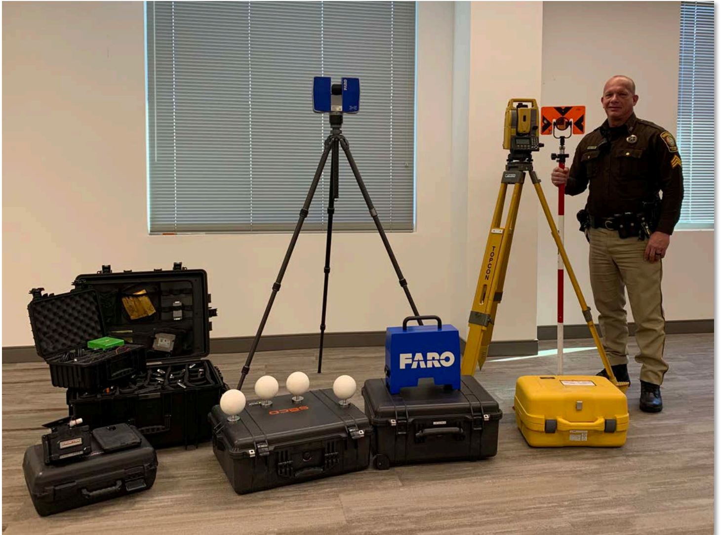
Sgt. Danny Beckworth poses with the Top Con and Faro laser scanner which uses laser technology to render a 3D model of a crash scene. The technology obtains information from a scene so that a forensic-scale drawing of the incident may be created. An auto-cad drawing program is used to create a scale drawing.
