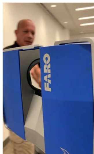
Sgt. Danny Beckworth poses with the Top Con and Faro laser scanner which uses laser technology to render a 3D model of a crash scene. The technology obtains information from a scene so that a forensic-scale drawing of the incident may be created. An auto-cad drawing program is used to create a scale drawing.
